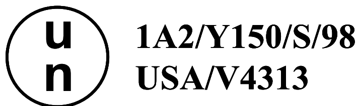
Figure 4-3. Sample United Nations specification marking.
