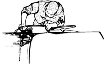
**STEP 2:** Drain plug: Ensure it is operable; it should be removable without excessive effort.
