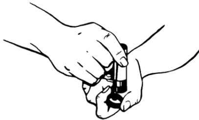
**STEP 4:** Hold the color comparator at eye level and toward a good light source.
