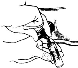
**STEP 3:** Place one chlorine test tablet in the comparator and allow it to dissolve.
